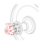
IMPORTANT: The indexing slot should be installed in the same position as noted in step 3.
